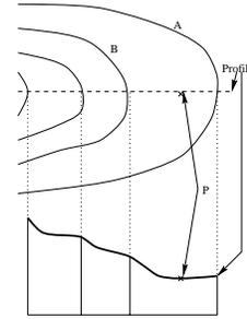
Figure 2: Profile (dark line) showing terracing problem in between contours
