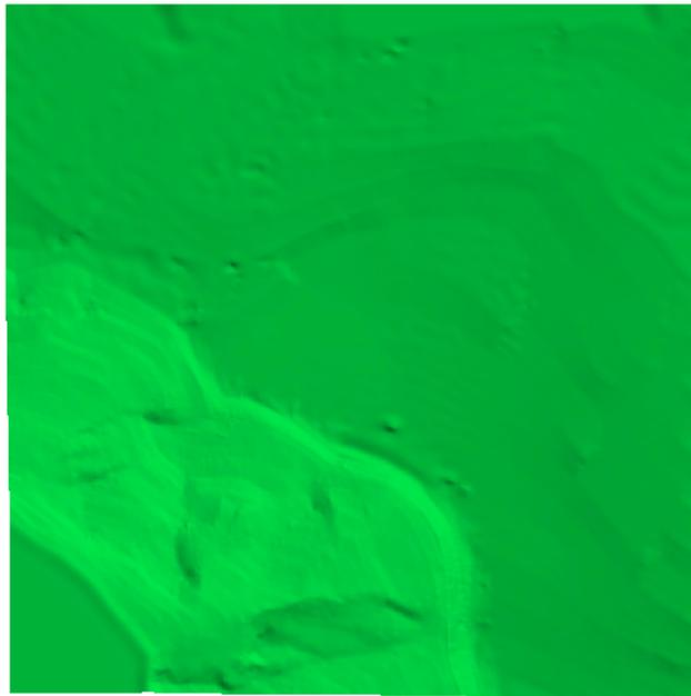
Figure 18: Crater Lake DEM obtained from gradient lines procedure
