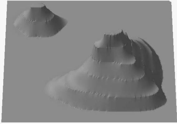
Figure 5: Thin plate under tension surface interpolation
