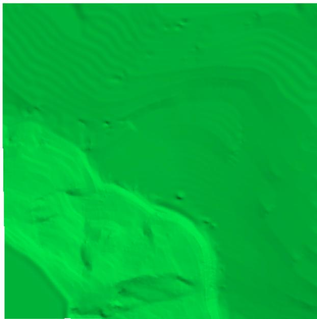
Figure 19: Crater Lake DEM obtained from intermediate contours and thin plate approximation
