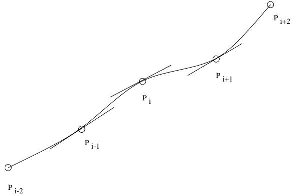
Figure 6: Catmull-Rom spline through contour elevations  $P$ . The straight line segments indicate the direction of the chord that connects adjacent points.
