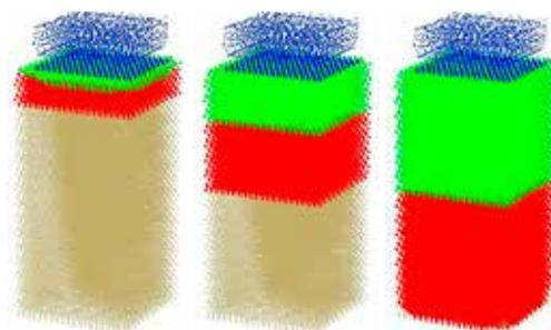
Figure 4. Permeability simulation result produced using proper  $\alpha$  and  $\beta$  values matched physical test result: particles were marked blue if above 78% saturated (top soil sample saturation), green if above 62% saturated (middle soil sample saturation) and red if above 32% saturated (bottom soil sample saturation)
