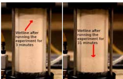
Figure 3. Physical saturation tests using soil and clay mixture
