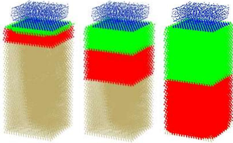
**FIG. 6. Permeability simulation result produced using proper  $\alpha$  and  $\beta$  values matched physical test result: particles were marked blue if above 78% saturated (top soil sample saturation), green if above 62% saturated (middle soil sample saturation) and red if above 32% saturated (bottom soil sample saturation)**
