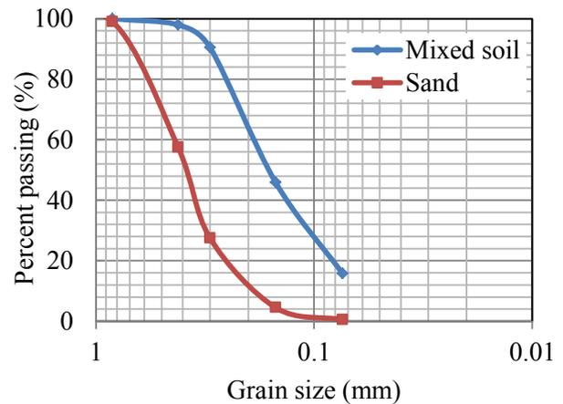
**FIG. 1. Grain size distribution curves of soils**
