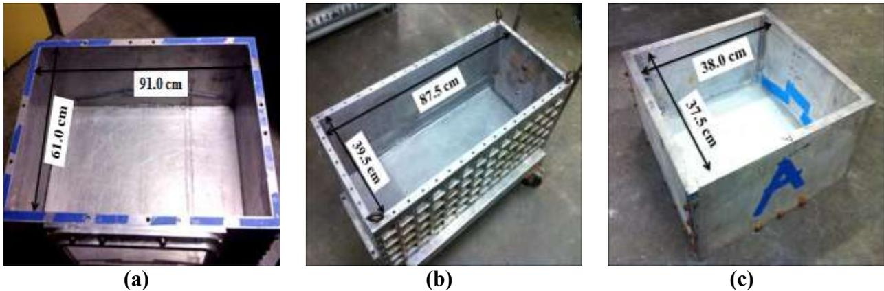
**FIG. 2. Aluminum model boxes (a). Big box, (b) Medium box, (c). Small box**
