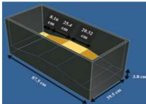
**FIG. 3. Dimensions of the modeled levee in the medium box**
