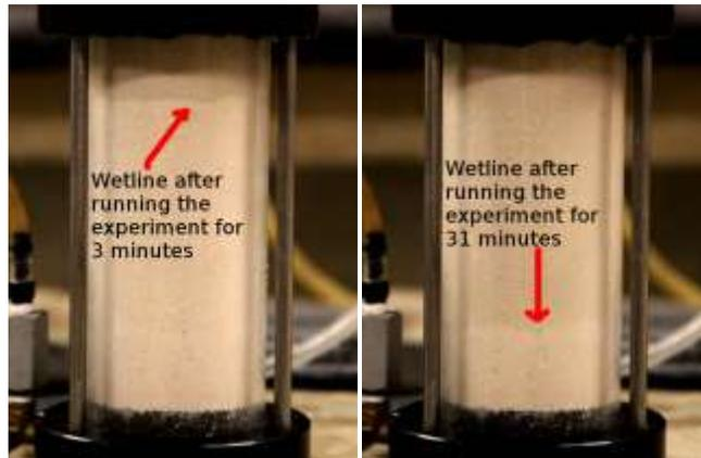
**FIG. 5. Physical saturation tests using soil and clay mixture**
