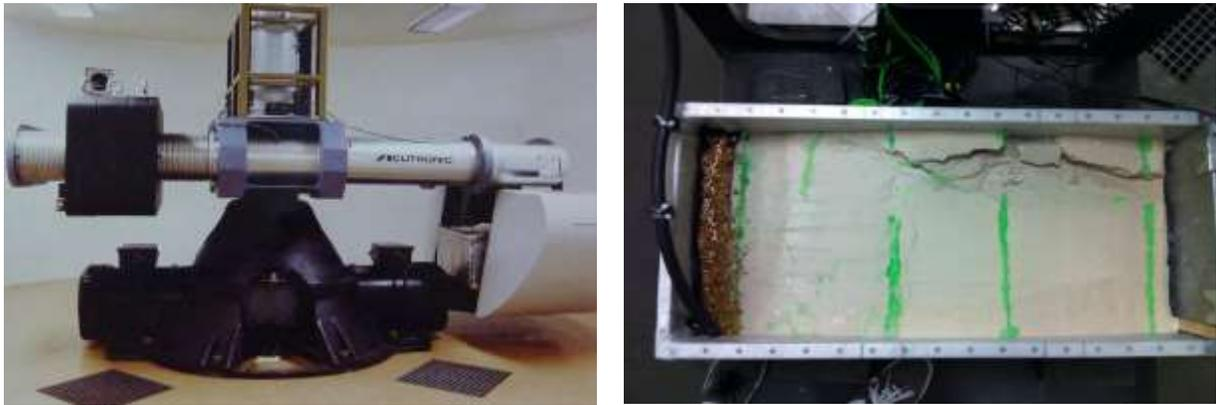
**FIG. 4. (a). RPI 150 g-ton geotechnical centrifuge, (b). The eroded levee after the centrifuge test**
