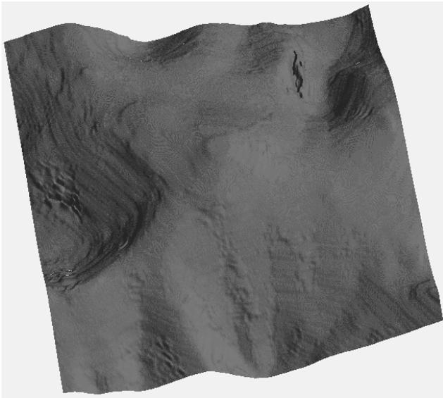
Figure 9: DEM computed with ArcInfo's TOPOGRID.
