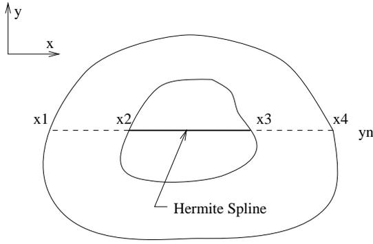
**Figure 3: Computation of peak area using Hermite spline**
